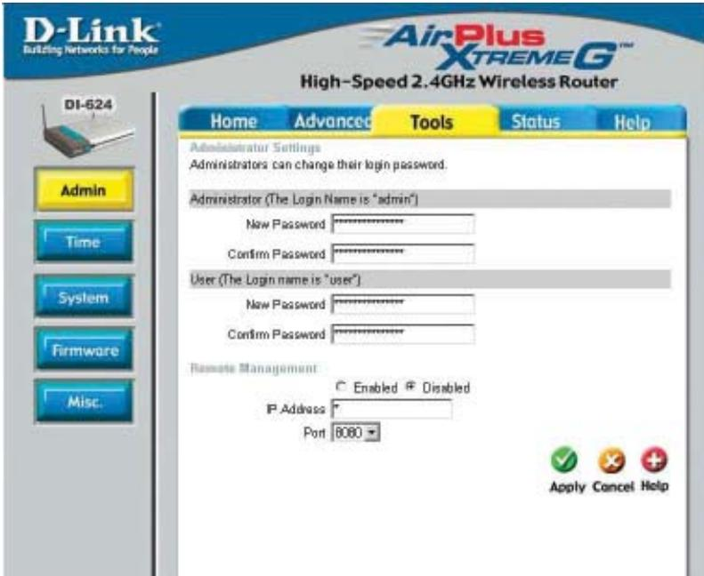
At this page, the DI-624 administrator can change the system password. There are two accounts that can access the Broadband Router's Web-Management interface. They are admin and user. Admin has read/write access while user has read-only access. User can only view the settings but cannot make any changes.
