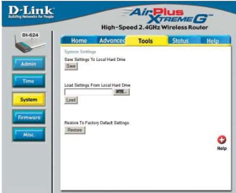
The current system settings can be saved as a file onto the local hard drive. The saved file or any other saved setting file can be loaded back on the Broadband Router. To reload a system settings file, click on **Browser** to browse the local hard drive and locate the system file to be used. You may also reset the Broadband Router back to factory settings by clicking on **Restore**.
