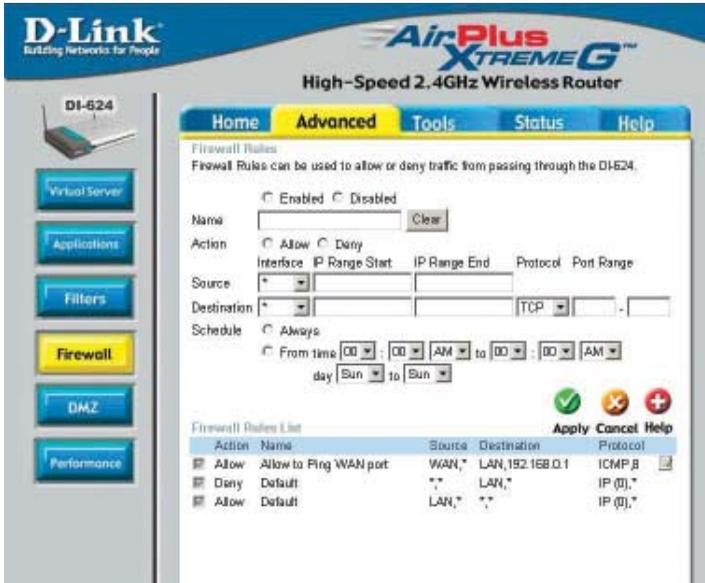
**Firewall Rules** is an advanced feature used to deny or allow traffic from passing through the DI-624. It works in the same way as IP Filters with additional settings. You can create more detailed access rules for the DI-624. When virtual services are created and enabled, it will also display in Firewall Rules. Firewall Rules contain all network firewall rules pertaining to IP (Internet Protocol).
