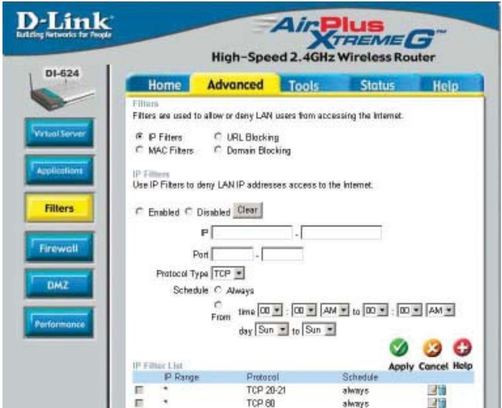
Filters are used to deny or allow LAN (Local Area Network) computers from accessing the Internet. The DI-624 can be setup to deny internal computers by their IP or MAC addresses. The DI-624 can also block users from accessing restricted web sites.
