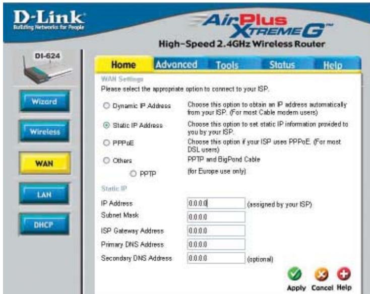
**Static IP Address-** Choose Static IP Address if all WAN IP information is provided to you by your ISP. You will need to enter in the IP address, subnet mask, gateway address, and DNS address(es) provided to you by your ISP. Each IP address entered in the fields must be in the appropriate IP form, which are four octets separated by a dot (x.x.x.x). The Router will not accept the IP address if it is not in this format.
