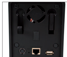
There's a lever at the back for each hard disk for easy ejection and removal
