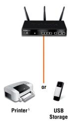
Supports one (DSR-250/250N/500/500N) or two (DSR-1000/1000N) USB 2.0 devices to extend functionality via D-Link's SharePort feature.
