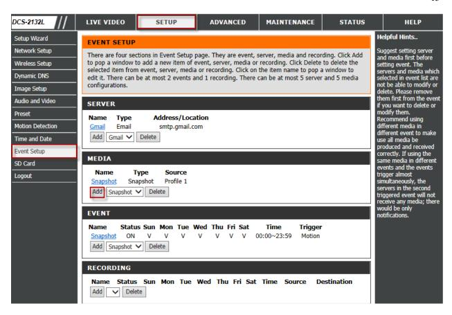
Step 6: Under the MEDIA TYPE section, configure the following; Select Snapshot
