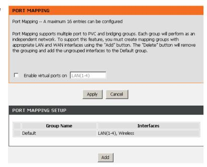
In this page, you can bind the WAN interface and the LAN interface to the same group. When you setup the port mapping, you need to enable the virtual ports at first.
